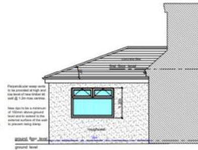
PROPOSED PART SIDE (EAST) ELEVATION. 1:50.
