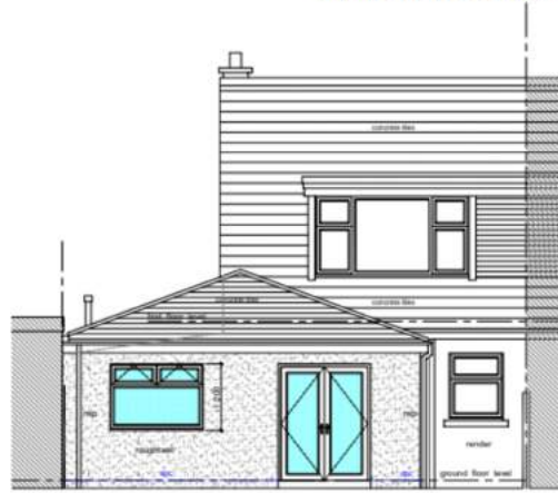
PROPOSED REAR (SOUTH) ELEVATION. 1:50.
